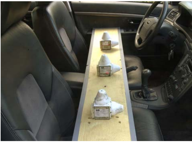
Fig. 2 Positioning of the electric field probes for measurements above the front seats
