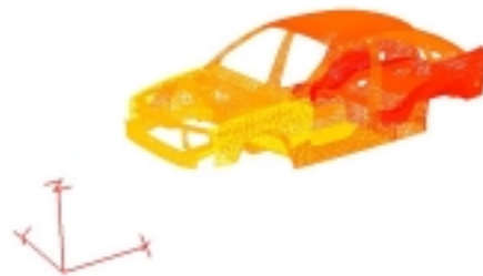
Fig 1. NEC mesh of the car
