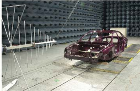
Fig 1: MIRA Semi Anechoic chamber: the antenna and the car
