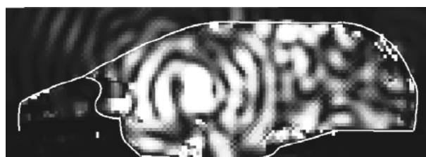
Figure 4: Fields generated by a transmitter located between two front seats
